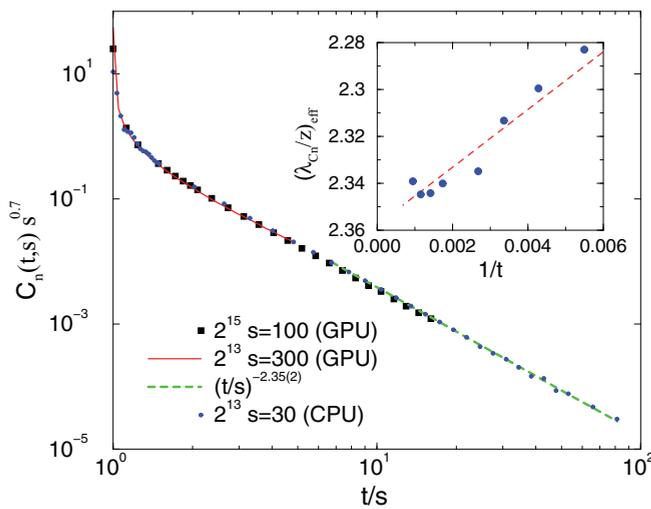
FIG. 4. (Color online) Autocorrelation function scaling of the lattice-gas variables for  $L = 2^{15}$ ,  $s = 100$  (boxes, GPU),  $L = 2^{13}$ ,  $s = 300$  (line, GPU), and  $L = 2^{13}$ ,  $s = 30$  (squares, CPU). The dashed line shows a power-law fit  $\sim (t/s)^{-2.35(2)}$  for  $t/s > 4$ . Inset: Local slopes of the  $L = 2^{13}$ ,  $s = 30$  data defined as (9). The dashed line shows a power-law fit.
