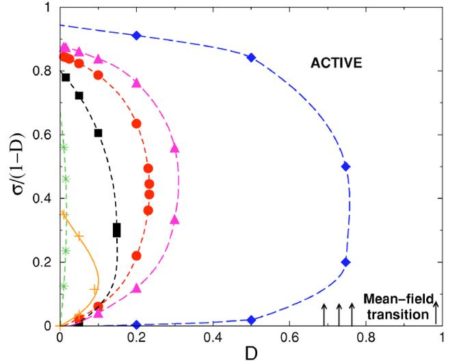
FIG. 1. Phase diagram of the  $2A \rightarrow 3A \rightarrow 4A \rightarrow \emptyset$  model. Stars correspond to  $N=2$ , boxes to  $N=3$ , bullets to  $N=4$ , and triangles to  $N=5$  cluster mean-field approximations. Diamonds denote 1D; + signs denote 2D simulation data, where PCPD class transitions are found. The lines serve to guide the eye. At the  $\sigma=0$  line, asymmetric, Eq. (5) type mean-field transition occurs.
