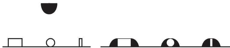
Figure 4.1: Illustration of the distortion arising due to tip-sample convolution effects for objects with different shapes. When the object becomes sharper than the tip, the object will generate the image of the tip. From [70].
