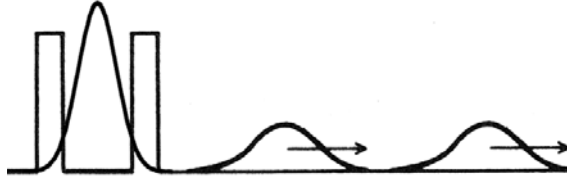
Figure 5.18: Sketch of a 1D resonant tunneling situation. Probability density is shown by a thick line. The quasi localized state in the double barrier region is decaying in distinct impulses.
